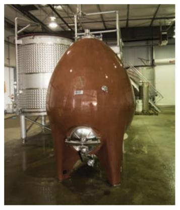
A concrete egg is used to ferment the Andis Cabernet Franc, preserving the flavors that come from a high-elevation volcanic site in El Dorado County.
