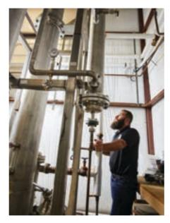
Western Son Distillery's products are ten-times distilled in a 20-foot column still. The process, which distiller Vinny Messina (pictured) calls the brand's "signature," ensures that the finished product tastes "as pure as possible."
